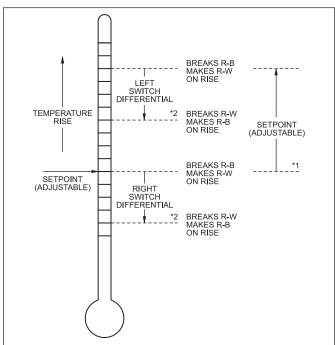
\*1 Difference between the temperatures at which the two switches make R-W. Adjustable from  $3^{\circ}$ F to  $10^{\circ}$ F ( $1.7^{\circ}$ C to  $5.6^{\circ}$ C) on standard models, or from  $3.6^{\circ}$ F to  $12^{\circ}$ F ( $2.0^{\circ}$ C to  $6.7^{\circ}$ C);  $55^{\circ}$ F to  $175^{\circ}$ F ( $13^{\circ}$ C to  $79^{\circ}$ C) models.
